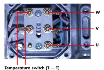
Previously, IBC used three-phase motors made by Gefeg. These motors are wired as illustrated on the left.
