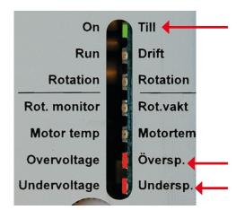
When both the Overvoltage and Undervoltage indicators are lit, it indicates overvoltage or a short-circuit.
