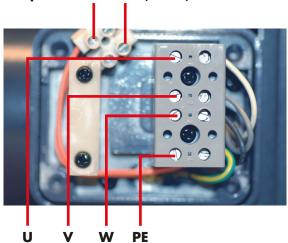
VVX motors with outputs of 25, 40 and 60 W are geared motors designed for 3x230 V. They cannot be rewired for 3x400V.
