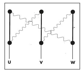
Tests should be performed using a Megger or a universal instrument to make sure that the motor windings are intact.
