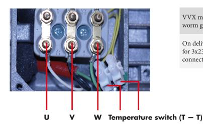
VVX motors with outputs of 90, 180, 370 and 750 W are worm gear motors designed for 3x230/400 V (Star/Delta).
